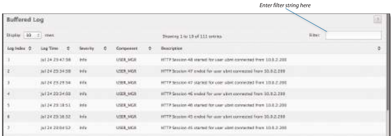
Filtering the Contents of a Table
